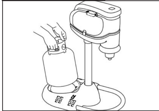
Step 1 - Propane Tank Placement
